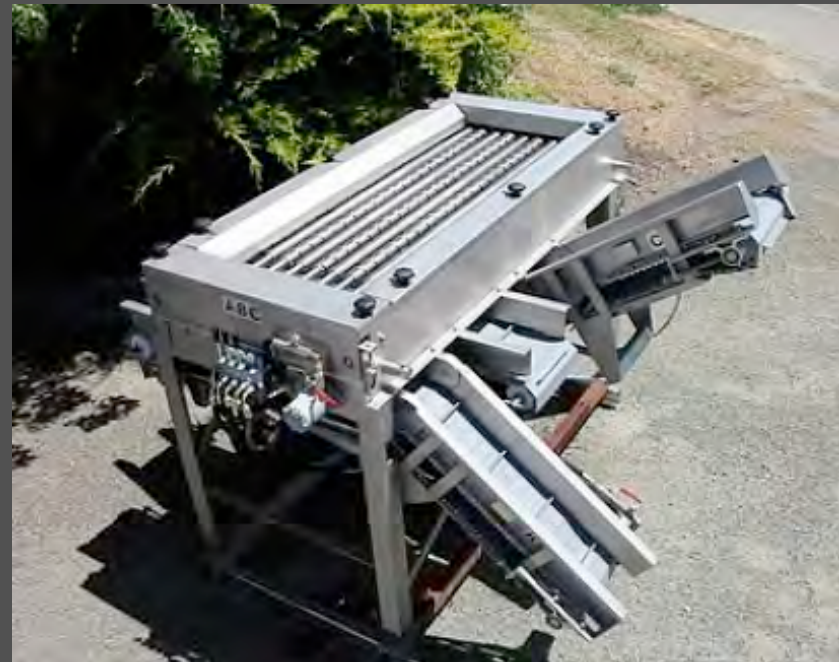
NZ Declumper and Grader Machines 2 to 3 tons per hour capacity
