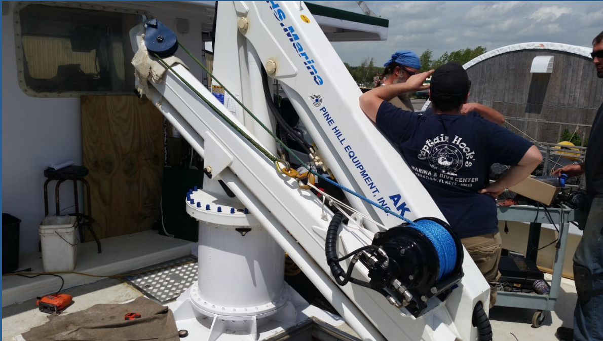
Crane and knuckle boom
